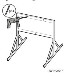
**Step 3** Align the rear panel with hole positions, insert M10x60 bolts into the holes, and tighten the bolts to a torque of 30 N m using a torque wrench, as shown in Figure 4-9.
