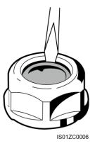
Figure 5-8 Installing a cable gland and adapter
