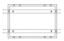
Maximum Load: Uplift load ≤ 2400 Pa Downforce load ≤ 2400 Pa
