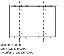
Compatible module types: CS3U-P, CS3U-MS, CS6U-P, CS6U-M and CS3W-P
