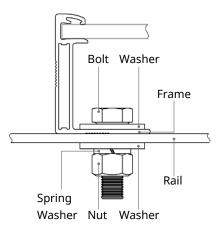
Modules should be bolted at the following hole locations depending on the configuration and loads: Table 3-1: Approved bolting methods
