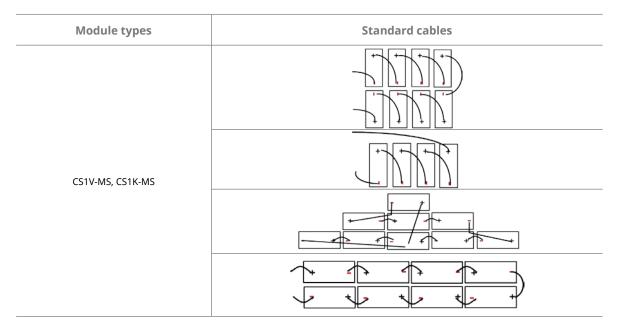
The maximum distance between two adjacent module frames should be within 50 mm (1.96in) for side with mounting clamps, and within 25 mm (0.98in) for side without mounting clamps, in order to meet system cable scheme.
