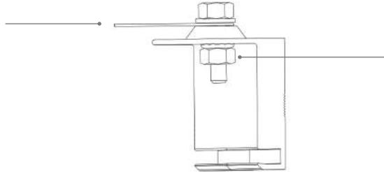
2. Then tighten the bolt using the toothed nut.
