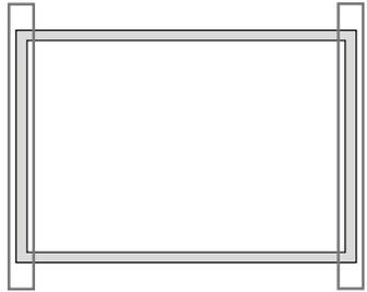
Use two insertion profiles running perpendicularly to the long side frame.
