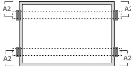
Use four clamps on the short side. Mounting rails run parallel to the long side frame.
