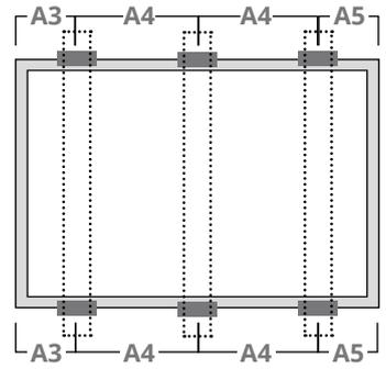
Use six clamps on the long side. Mounting rails run perpendicularly to the long side frame.
