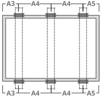
Use six clamps on the long side. Mounting rails run perpendicular to the long side frame.
