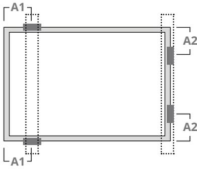
Use two clamps on the long side and two clamps on the short side. Mounting rails run perpendicular to the long side frame.
