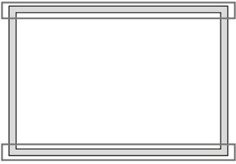
Use two insertion profiles running parallel to the long side frame.
