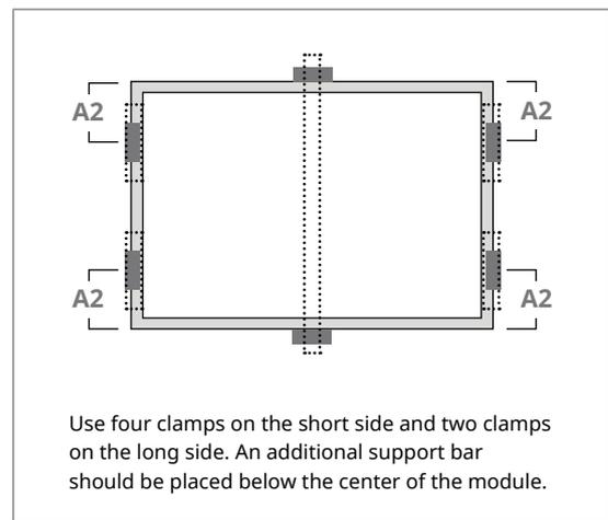
Use four clamps on the short side and two clamps on the long side. An additional support bar should be placed below the center of the module.
