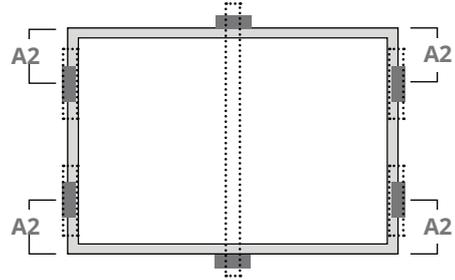
Use four clamps on the short side and two clamps on the long side. An additional support bar should be placed below the center of the module.
