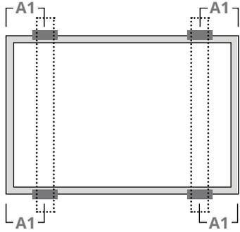
Use four clamps on the long side. Mounting rails run perpendicular to the long side frame.
