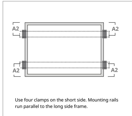
Use four clamps on the short side. Mounting rails run parallel to the long side frame.
