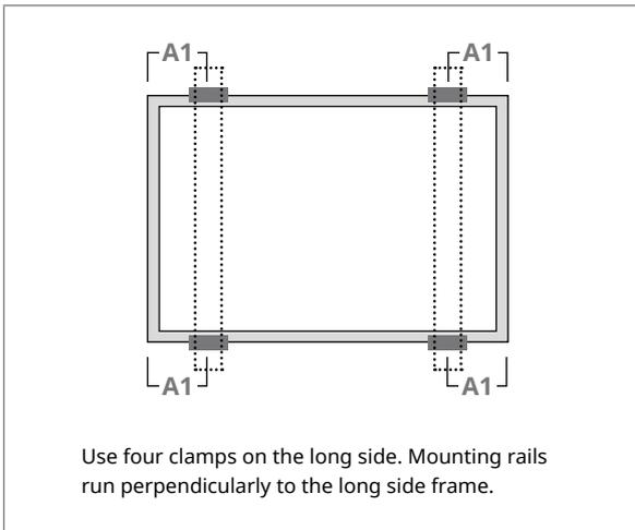
Use four clamps on the long side. Mounting rails run perpendicularly to the long side frame.
