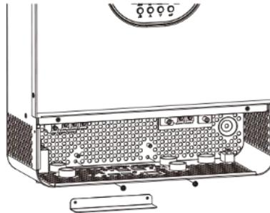
**Step 5:** Install new parallel board with 2 screws tightly.
